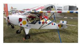
The mystery aircraft to the left is a **Belite Superlite**. an American single-seat, high-wing ultralight aircraft developed from the Kitfox Lite James Wiebe in 2011. The fuselage is made from 4130 steel tubing. Flaperons and vortex generators are used to improve roll control and low speed flight. The wings are foldable for storage. A Belite aircraft was used in Mythbusters episode 174 – Duct Tape Plane which successfully flew after repairing skin tears with duct tape.
