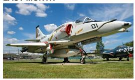
Last month's picture was a **McDonnell Douglas A-4M Skyhawk II**, a single-seat subsonic light attack aircraft. It was used by the US Navy and US Marines in the 1950s as a replacement for the propellor-driven Douglas A-1 Skyraider. The Skyhawk has a short-span delta wing configuration, a tricycle undercarriage, and is powered by a single turbojet engine.
