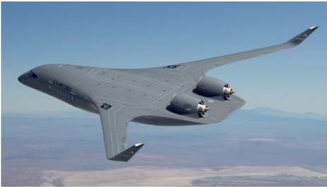
The mystery aircraft to the left is an artistic concept of a blended-wing body (BWB) aircraft. In August 2023, JetZero was selected by the U.S. Air Force to build a demonstrator aircraft with a BWB design. JetZero's BWB will be a full-scale demonstrator, as the program's solicitation specifically called out applications for tanking, cargo and even commercial tasks.
