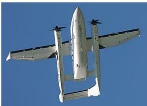
The mystery aircraft to the left is a **Sukhoi SU-80**, a Russian twin turboprop, twin boom STOL transport aircraft. The prototype first flew in September, 2001.
