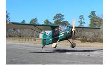
It is a Zippy Sport LSA designed by Ed Fisher and marketed by Green Sky Aviation. The Zippy Sport is a single-seat, high-wing monoplane powered by a 50 hp (37 kW) Rotax 503 piston engine. Other engines have been fitted, including VW. Of mixed construction, it has a welded 4130
