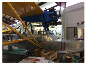
It has a very early adjustable pitch propeller and the smallest two-row radial engine ever-built; a 165 hp, 6 cylinder Curtis "Challenger".
