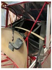
As well he had started a full sized Great Lakes. It has wing ribs, a Kinner radial engine and a prop. The fuselage has been welded. The tail feathers are complete. The firewall is loosely mounted. He has mounted some instruments and the panel is mounted in the fuselage.
