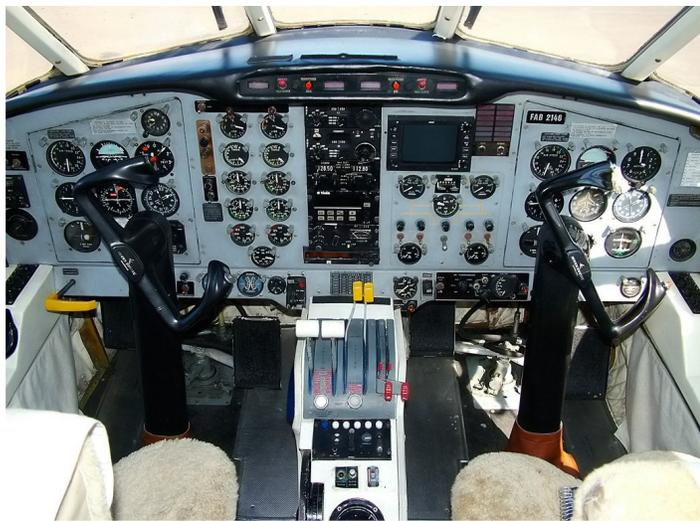
Bandeirante flight deck with steam gauges and a weather radar display screen (Wikipedia photo)
