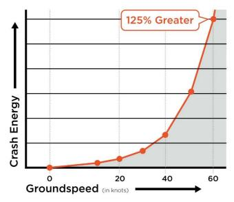
ground or water the gear might dig in and cause the airplane to flip over. On the other hand, it might absorb some of the energy of a crash, or help stop the aircraft if space is limited.
