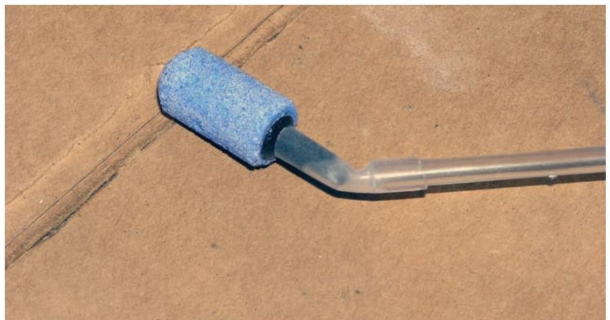
The engine dryer system consists of a vibrating air pump, a two-liter plastic pop bottle, an airstone aquarium air bubbler as a filter, plastic tubing and silica gel pellets to remove moisture. It can be attached via the oil filter port or by way of the crankcase vents.
