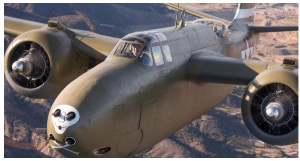
Lewis' Havoc was built in 1943 as an A-20G, is powered by two 1,700-hp Wright R-2600s, armed with seven 7.7mm (.303 caliber) machine guns (six Brownings, one Vickers) and could carry a bomb load of 4,000 pounds. The airplane was previously owned by the Lone Star Flight Museum, but has since been fully restored to its original, stock military configuration. AirVenture Oshkosh 2016 is expected to be the A-20's first official public display since the restoration.
