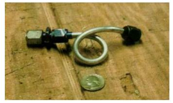
when finished. Then install the sleeves and nuts and flare the tubing ends. Then install unions on both ends and cap one end with an AN 929 cap. Fill the tubing completely with bead blast material (sandblasting sand will work) andcap the other end with the
