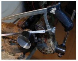
WHEN THE NEED ARISES to cut off a section of pipe or tubing, especially if the diameter is larger than 1 inch, it can be difficult to keep the cut square with the length of the tube. If you place a hose clamp around the tube at the cut line, you will create a very solid line that is perfectly square with the tube and substantial enough to act as a cutting guide for your saw. In the photo a piece of 3-inch diameter thin wall tubing is easily cut perfectly square with a hacksaw.
