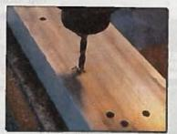
9. Drilling out flush rivets uses the same process. After center-punching the factory head, start the drill slowly and drill down just until you reach the shank.
