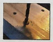
3. Start the drill with a few short, slow pulls of the trigger; the idea is to center the bit in the dimple before starting to really drill. Once you start drilling, make sure you actively steer the bit into the center of the rivet head.
