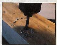
11. If you have perfectly centered the drill bit, the remains of the head might just climb the bit itself. In either case, pop the remains of the shank and shop head out the back side and get on with your build.
