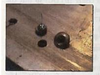
8. If you do a clean job removing the rivet, you will be able to keep the shop and factory heads as souvenirs. (Unfortunately, even the best builders have quite a collection of drilled-out rivets, so they won't fetch much money on the collector's circuit.)
