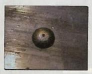
1. The factory head on this universal-head rivet is fine, but the shop head wasn't up to spec, so out it comes. Note the dimple in the center of the head; this can be enough for experienced builders to use to center their drill bit.
