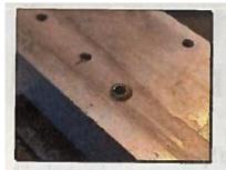
4. You aren't trying to drill all the way through the rivet shank—just deep enough to separate the head from the shank. If you feel that you are drilling into the surrounding material, stop!
