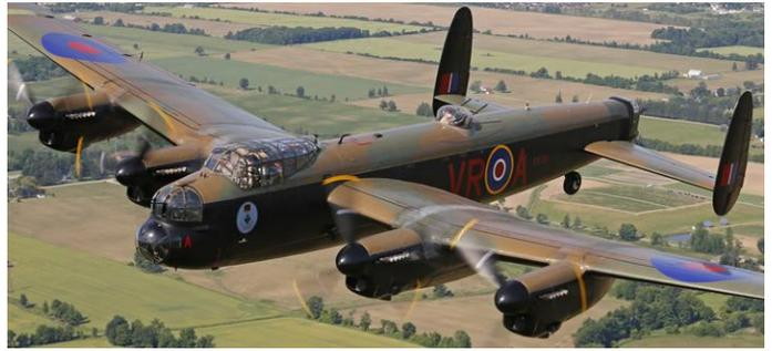
Powered by four Packard-built Merlin engines, the Lancaster was the only Allied bomber capable of carrying and delivering the 22,000-lb. "Grand Slam" bomb. Lancasters measure 69 feet, 6 inches with a 102 foot wingspan. Its four 1640 hp Packard Merlin 224s propel the plane to a maximum speed of 275 mph.
