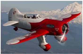
from the original Granville brothers design. The Cyclone, as Moss stated in Sport Aviation, was the same diameter as the Pratt with twice the horsepower (1,425 vs. 675). To account for the Cyclone's 200-pounds of extra weight, Moss reduced the fuel tank from 480 gallons to 240 gallons.
