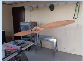
Finished copy of Mini Coupe Propeller
