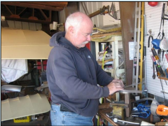
Here he's building a baffle trim piece for his Nieuport using a metal shrinker.
