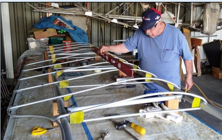
Here he is checking his work. Wing structure is completed. Now on to all the minor little details, like ailerons, skin on the leading edge, boxed in aileron bay, control rigging, etc., etc.
