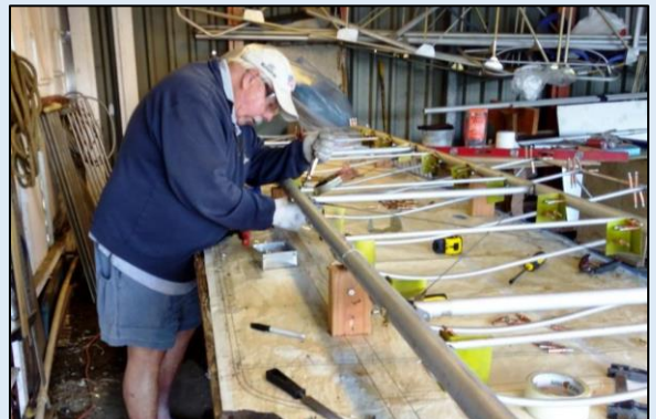
Talk about progress! The top ribs are done and clecoed together. Wing has been flipped over and placed on blocks that were shot in with a transit ensuring that when the actual riveting takes place the wing will remain as flat as possible. Jimmy is now working on the bottom half of the split ribs.
