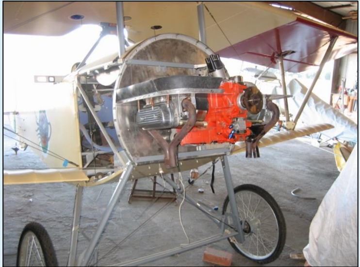
This is the preliminary mounting of the engine with a good look at the sharp looking baffling.
