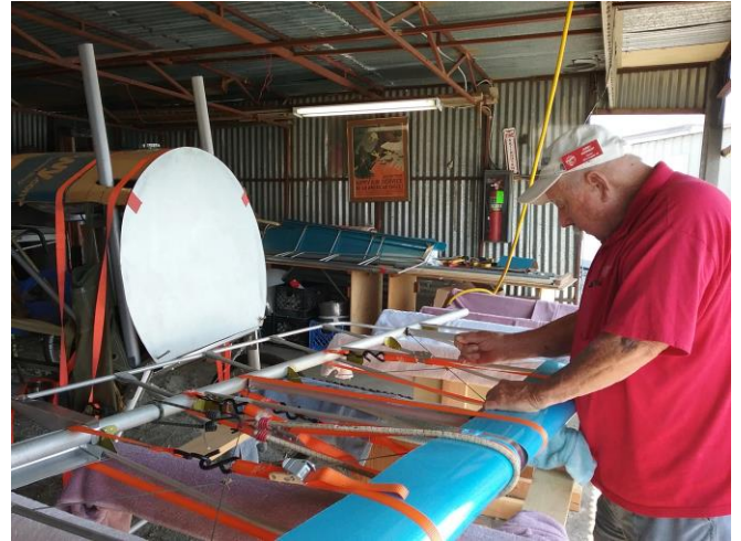
Jimmy Kennedy rivets the leading edge cover onto his Nieuport. 4/27
