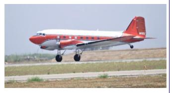
Turbo DC-3 seen at Brown Field. This one is owned by Basler Turbo Conversions, the company that re-engined the plane. They call it a BT-67 but to the FAA, it's still a DC-3.
