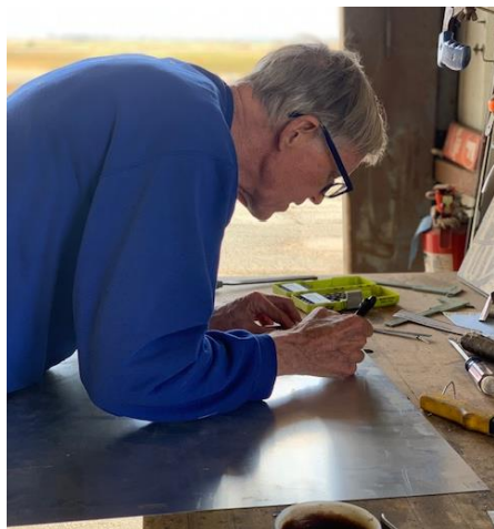
Jim MacKinnon lays out a sheet aluminum part for his Nieuport.
