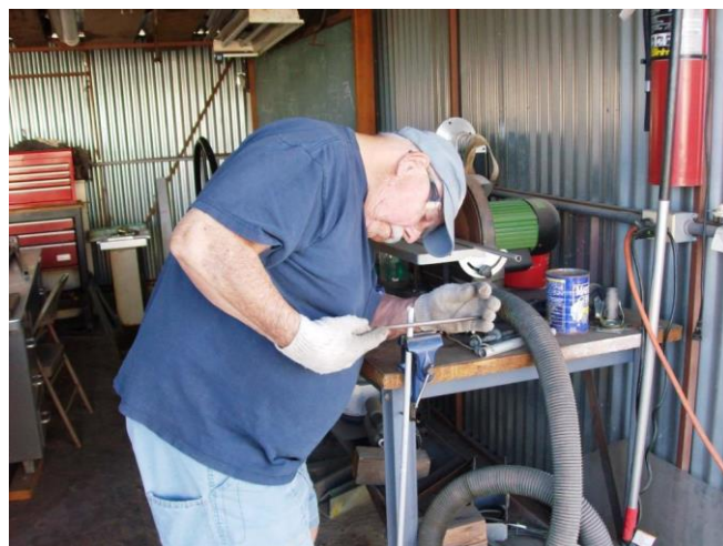
Now if we can just wake him up! Actually, Jimmy is carefully coping the end of a rib to fit around the spar.
