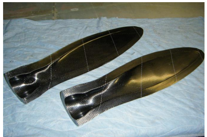
Female molds created from the male blanks
