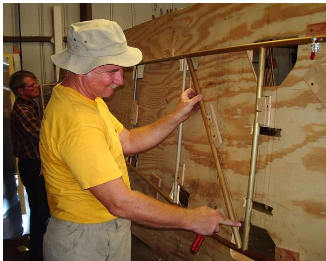
Gene Hubbard (r) and Richard Kalling fit tubes in the Nieuport fuselage jig.
