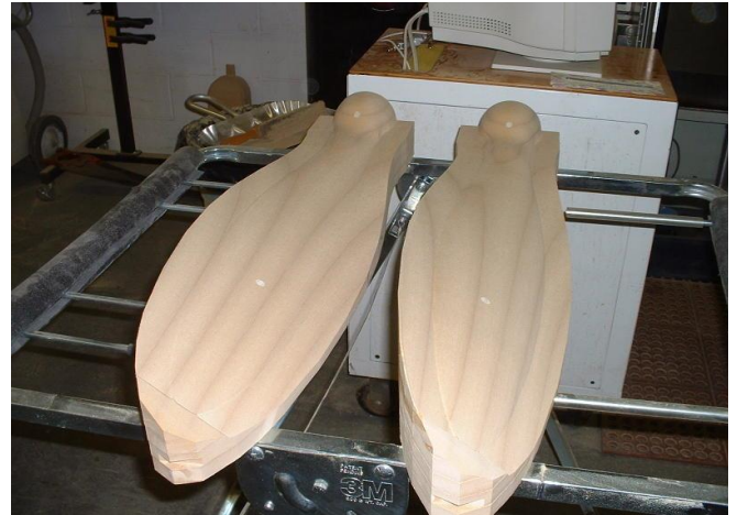
The male "blanks" for the propeller, front and back sides
