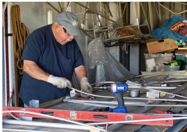
The Nieuport wing uses split ribs. Here Jimmy fits the top half of a rib to the wing frame.
