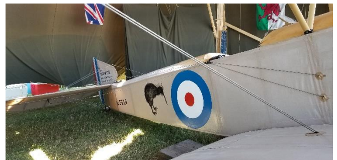
Aft Fuselage: Wires everywhere. This one is in British markings, but most of the 6,000 or so 1 1/2 Strutters built were actually flown by the French. The Russians, Americans, Belgians, and Japanese also flew them
