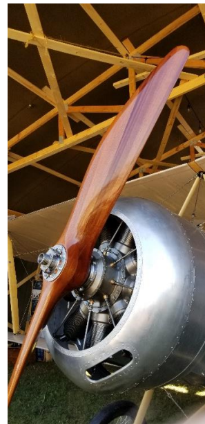
KIP Aero's replica of the Sopwith 1 1/2 Strutter. This was a two-seat fighter that saw service in WWI in the 1916-1917 time frame. The replica uses a real rotary engine. If you have to ask how much it costs, either in kit form or assembled, you can't afford it!
