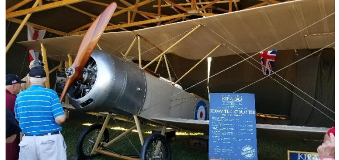
KIP Aero's replica of the Sopwith 1 1/2 Strutter. This was a two-seat fighter that saw service in WWI in the 1916-1917 time frame. The replica uses a real rotary engine. If you have to ask how much it costs, either in kit form or assembled, you can't afford it!
