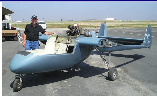
Ryan shows off the O-200 engine conversion on his Sparrowhawk.
