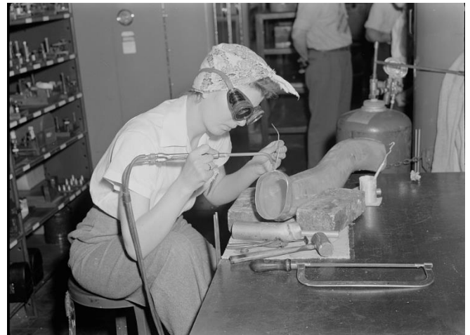
A woman at the Willow Run plant welds parts of the cooling system on a supercharger. July 1942
