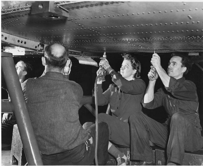
Riveting a center wing section for a B-24E bomber in the horizontal position at Ford's Willow Run plant, February 1943.
