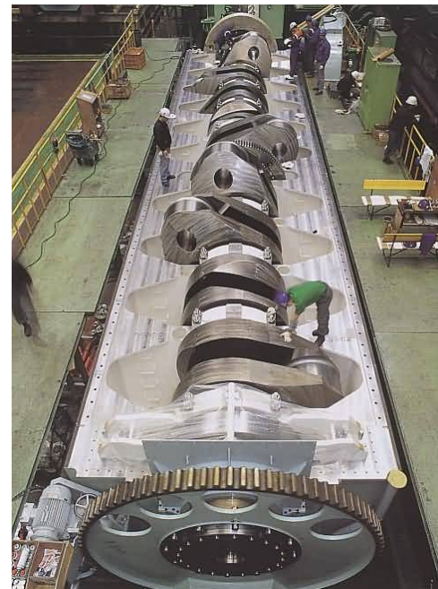
Crankshaft of the 'smaller' 10 cylinder version
