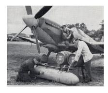
A staged shot of the Mod. XXX tank being filled.
