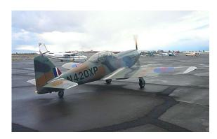
Vern bought the aircraft in 1997 as a partially constructed two-place tandem plans kit and spent the following fourteen years completing the project---he finally had his first flight in 2010! It holds 60 gal of fuel with a burn rate of 12-13 GPH, a cruise speed of 210 MPH, an empty weight of 1,860 lbs. and gross of 2,600lbs. It is currently for sale with an asking price of \$250,000.00 and total tach time of 37 hrs.
