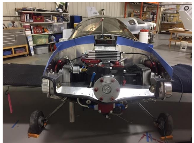
Big frontal view of Dale's new, 100 hp, Turbocharged VW engine
