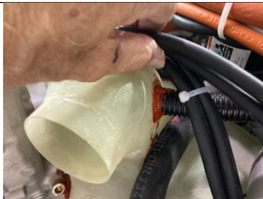
Blast tube to direct cooling air was installed
