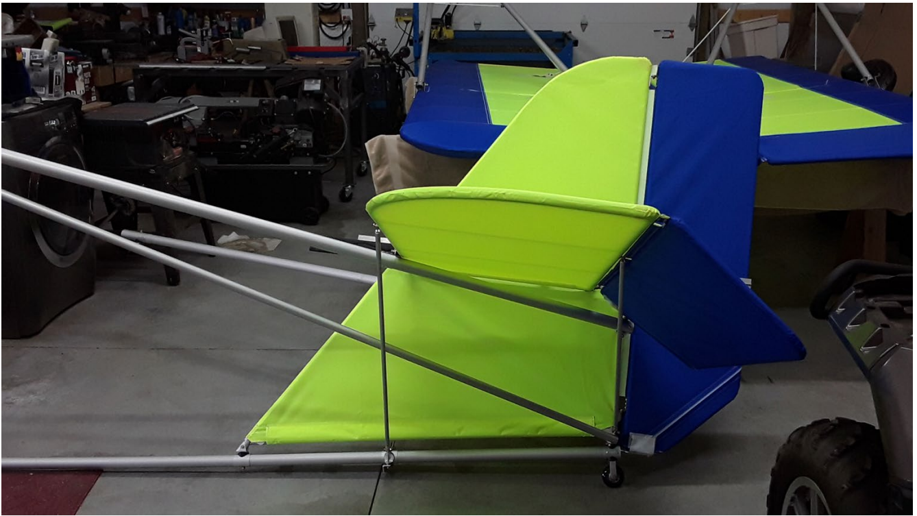
Completed tail section with rudder, elevator
