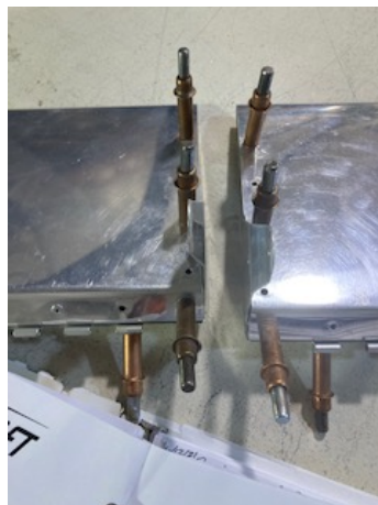
Drilling out the trim tab rivets
