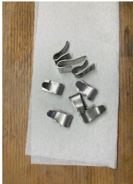
Fabricated door dogs that will be mounted on the doors for the door latches
