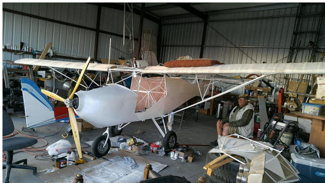
Charlie and Henry's Avid Flyer is 'close to being done'; now finishing wiring, brakes and fuel lines.
