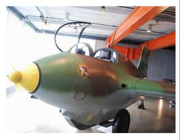
The Komet was a rocket-propelled fighter, built specifically to destroy high-altitude bomber planes. Unfortunately, its fatal flaw was its Walter rocket motor, which had a tendency to explode mid-flight. It was, however, a breakthrough in technology at the time. The model seen here is only one of a dozen Me-163 fighter planes left in existence.
