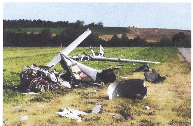
A fatal LSA aircraft accident resulting from improperly fastening the elevator control rod quick disconnect. Courtesy of the NTSB.
