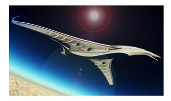
With an aerodynamic, bird-like design, the Stratoliner achieves maximum efficiency by utilizing oversized wings that allow the jet to generate enough lift to fly at very high altitudes. In addition, four Cryogenic Hydrogen Turbofan engines power the Stratoliner allowing it to fly massive distances while operating in a lower-power state with zero emissions.
