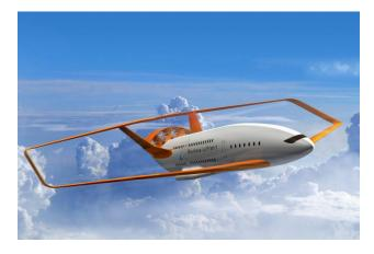
The "Claire Liner" (Claire = CLean Alr Engine) design concept utilizes a so-called Boxwing design. Known for its great stability, the concept has been around since the twenties and has already been used in model aircraft and ultralights.
