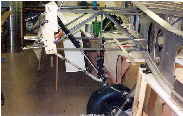
The main gear retracts just like the real B-17, and has proven to be the most complicated part of the project.
