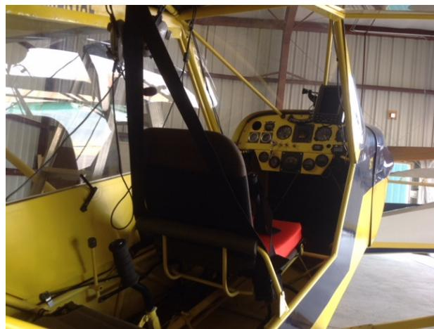
It's a very low time plane, hardly any on plane and a touch over 100 on motor. It's the early solid lifter Jabiru 2200 so it doesn't have the thru-bolt problems some of the later hydraulic lifter ones did. Good motor.
