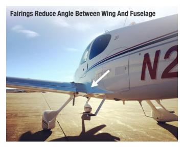
But interference drag isn't just limited to where the wings and fuselage meet. A Cessna 172 wing strut, for example, has fairings around the base and top of the strut, where the strut meets the fuselage and wing. Without fairings, these connections form noticeably acute angles, significantly increasing interference drag.
