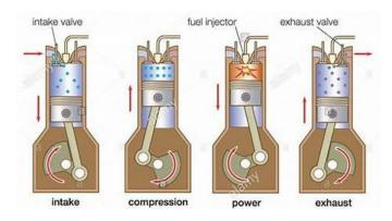
As a piston travels up in the cylinder it reaches "Top Center" about 8 degrees before reaching "Top Dead Center." The piston then travels down in the cylinder to "Bottom Dead Center."
