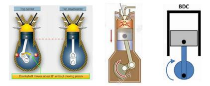
An engine does "useful work" when it produces power by igniting the proper fuel/air mixture at the proper time. Therefore, our discussion will center on the "Power Stroke."
