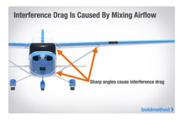
As air flows around different aircraft components and mixes, it needs to speed up in order to pass through the restricted area. As the air speeds up, it requires extra energy. At the same time, it creates turbulence, resulting in an increase in drag. The more acute (sharp) the angle, the greater the interference drag that's generated.
