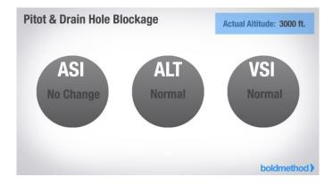
This will cause your airspeed indicator to show a faster-than-normal airspeed as you climb. It will also cause it to indicate a slower-than-normal airspeed as you descend. This can be a very disorienting sensation, especially in instrument conditions.
