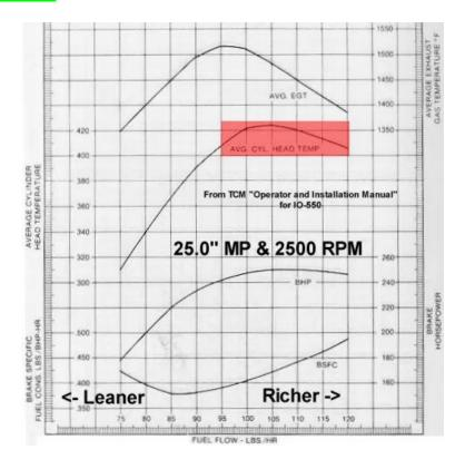
The high temperatures are the direct result of pulling the MP back to 25", which cuts out the power enrichment feature of the fuel controller, leaning the engine dramatically!
