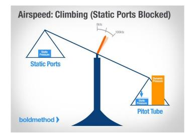
A static blockage will cause your airspeed indicator to show inaccurate indications. If you climb at a constant airspeed, your ram pressure's static component decreases. Since your static ports are clogged, they have too much static pressure. Essentially, they're stuck at a lower altitude. The difference between ram and static pressure is smaller, and your indicated airspeed decreases. You're now flying faster than your indicated airspeed. The opposite is true if you descend.
