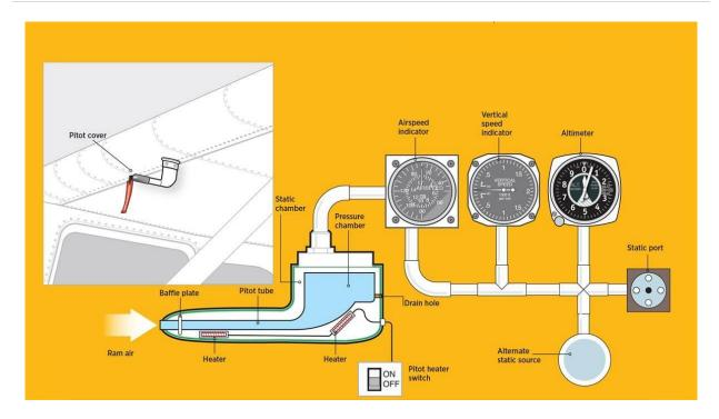
The airspeed indicator is the only instrument in the pitot-static system that uses both types of air pressure.
