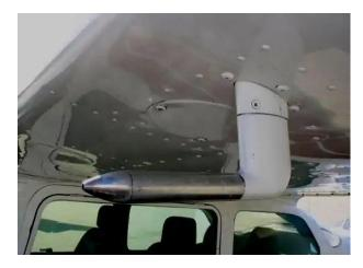
The pitot tube is usually mounted on the wing of the airplane so that it faces into the relative wind. A small hole in the tube allows impact air pressure—also known as ram air pressure—to enter.
