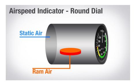
The only instrument connected to the pitot system is the airspeed indicator. For this explanation think of the airspeed indicator in simple terms. There is a diaphragm that has ram air pressure (from the pitot tube) on one side, and static pressure (from the static port) on the other side.
