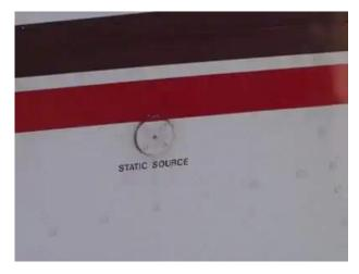
The static ports are attached to the airplane's fuselage
