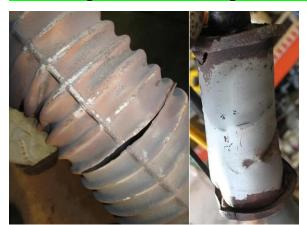
Exhaust system leaks are the most common cause of CO poisoning in GA aircraft, and the spot detectors (printed cards treated with a chemical that changes color in the presence of high CO concentrations) long used to monitor for dangerous cabin conditions do not produce aural alerts, and the visual cue is easy to overlook.
