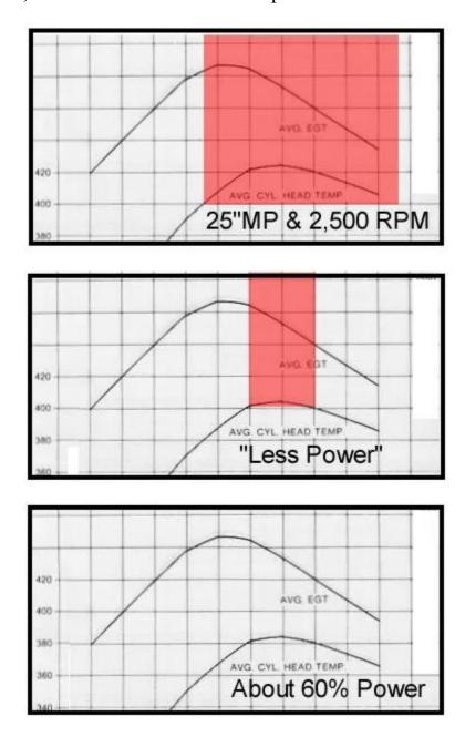
In the **second picture**, I've fiddled the CHT numbers, and erased the EGT numbers, to give a **simple picture of the engine operating at setting which is producing "Less Power."**
