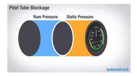
If your pitot tube becomes blocked, there is no more ram pressure entering the tube. Any excess pressure leaks out of the drain hole, and you'll be comparing the drain hole's pressure and the static pressure. This means your airspeed indicator will be at zero, just like when you're sitting on the ramp.
