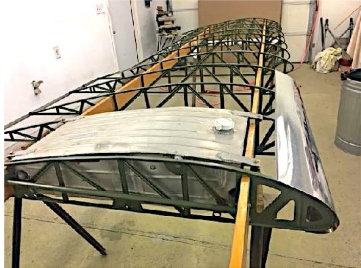
I also installed a 12-gallon wing tank in the left wing that feeds into the 12-gallon fuselage tank by opening a valve
