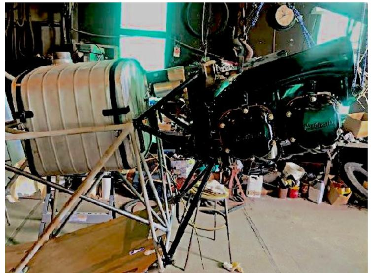
I added Grove disc brakes, a C-85 continental engine in place of the original Franklin that was long gone. Also installed a B&C light weight starter along with a Lithium-ion light weight battery.
