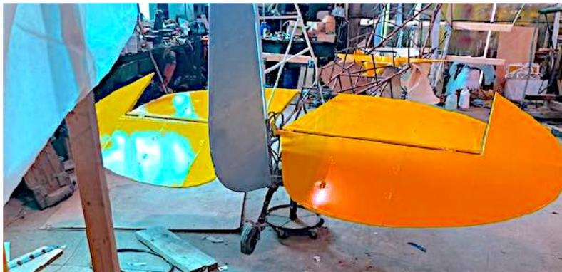
I used tri-pacer horizontal stabilizers and balanced elevators
