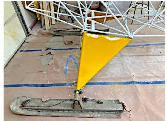
This jack assembly is used to stretch the bungy cords to install them on the landing gear.
