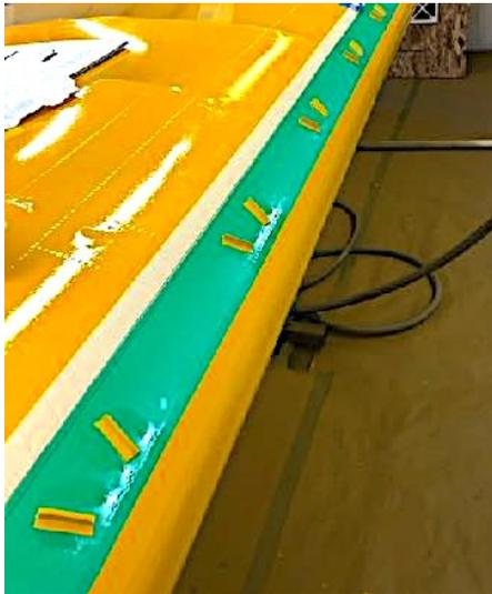
Added Vortex generators on the wings and horizontal stabilizer to reduce the stall speed
