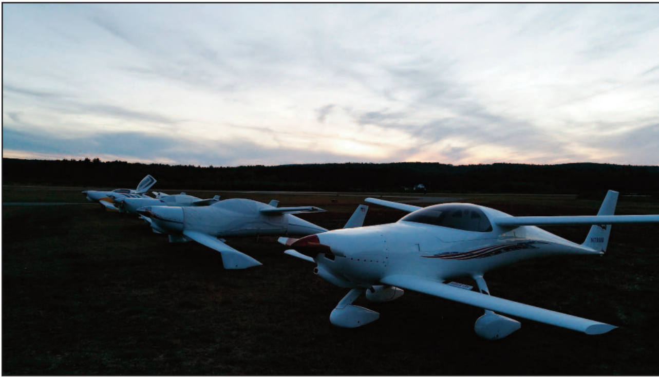
All the Quickies lined up at sunset. The foreground plane is a modified Quickie with tricycle landing gear. This variation is called the Tri-Q.
