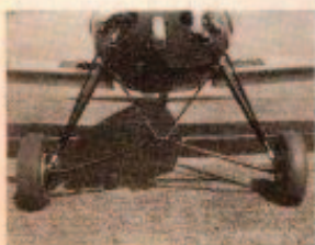
Another type of tubular landing gear developed by Consolidated for a 3-place job—a particularly good chair, built only in limited quantity.
