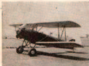
Latest type "Fleet" trainer. This type of tubular landing gear weighs only about 40 lbs. At 150 in service, no failures have occurred.
