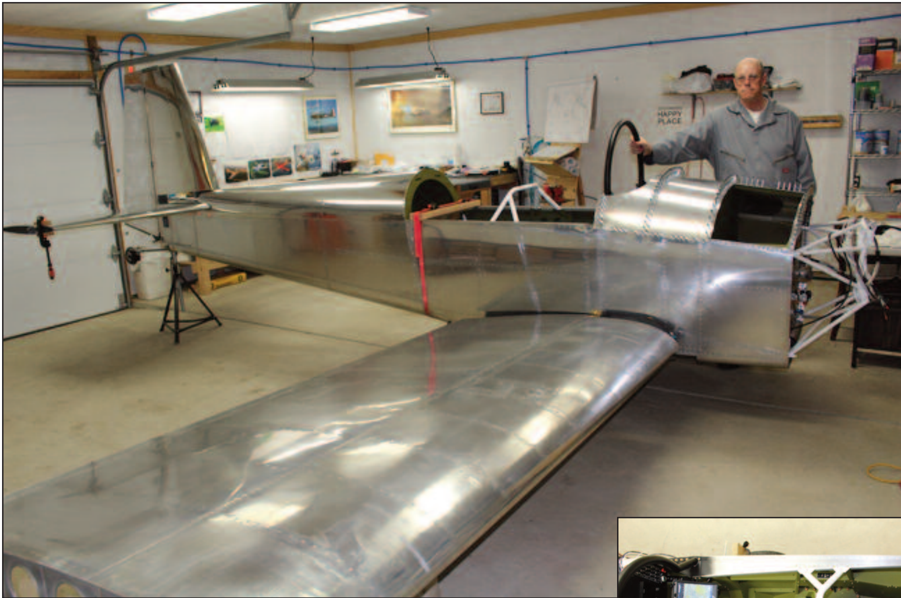
Wing fitted into place.
