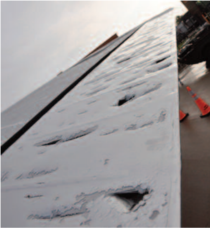
B-17 hail damage Wider view shows expensive damage to the right aileron.
