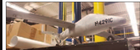
Below: Model of Prof. Leshner's TEAL for tunnel testing.
