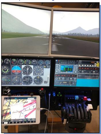
The second CPU running the visuals enables a more fluid and realistic experience. In addition, I can run Foreflight on my iPad mini connected to X-Plane just as if it were in a real aircraft.
