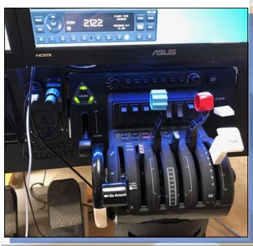
I will enclose pictures but the way this is all used is by running Windows 10, X-Plane 11, and Air Manager. The two CPUs are networked together so that one runs the flight and the other runs the visuals. The touchscreens have the flight instruments and navigation. using Air Manager and the Knobster I have realistic use of the instrument panel including the GPS.
