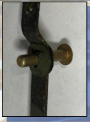
My old indicator with 10,000 hours of wear on it would not have lasted much longer. The new indicator will be an AN4 rivet like the original, but with two 80 year old Tinnerman Nuts to hold it in place. A little knowledge of old aircraft production techniques helped me to come up with an elegant solution to a curious problem!
