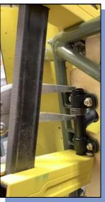
Now you can start the nuts, and tighten them only to the point where the springs can still do their job of pulling the pedals forward and tensioning the rudder cables. This has been a tedious, yet satisfying task!
