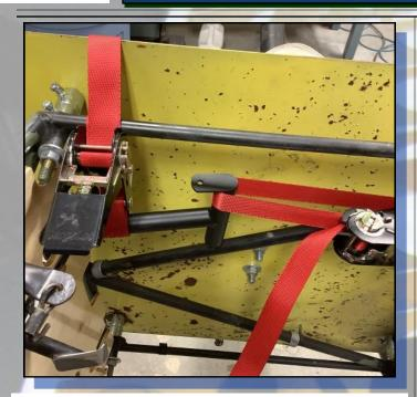
enough. Next place the pony clamp on the inboard stub of the pedal (under the floor) and pressure the pedal toward the spring side. You will find it necessary to also compress the spring with a vise grip to finally be able to install the second clamp half!
