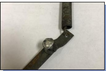
My first thought was to replace the rivet with a Rube Goldberg mash up of 4/40 machine screw, brass sleeve, washers, lock washers, etc. This just sounded too complicated, and too heavy. Those tenths of ounces build up in any airplane.
