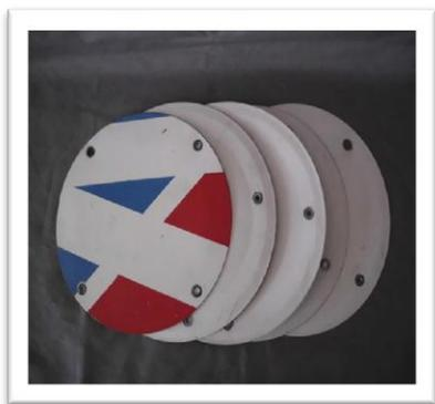
This is an example of the typical circular inspection panel covers found on Pipers or Cessnas. Usually these are held in place with sheet metal screws and are not intended to be part of the structural design
