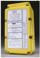
The FCC said the rule was designed to enhance the ability of search-and-rescue personnel to locate and bring aid to the victims of airplane crashes by accelerating the switch to the newer 406-MHz technology ELTs that transmit a digital distress signal with a variety of information identifying the beacon and the nature of the emergency, and sending out a homing signal.
