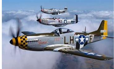
model, and transformed the aircraft's performance at altitudes above 15,000 ft (4,600 m) (without sacrificing range),<sup>[8]</sup> allowing it to compete with the <u>Luftwaffe</u>'s fighters.<sup>[9]</sup> The definitive version, the <u>P-51D</u>, was powered by the <u>Packard V-1650-7</u>, a <u>license-</u> <u>built</u> version of the two-speed, two-stage-<u>supercharged Merlin</u>
