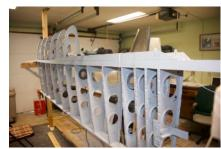
looked alike. Thank God for the numbering system of the parts by SPA. Measuring for square and level on the jig was a challenge. I am glad I had the factory build the main spars and fuel tanks as it would have increased my building time a few months.
